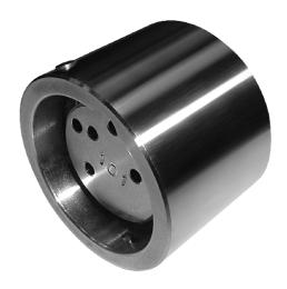
The HD Series SA3 Switchgear Adapter Interlock has a 5/16" (8mm) square, 3/8" (9.5mm) long shaft that is controlled by the robust HD Series key. The SA3 is attached to the interlock provisions by way of (4) 10-32 tapped holes in the bottom of the lock cylinder. The interlock can be ordered with the shaft rotating clockwise or counterclockwise. Multiple degrees of rotation are available also.
